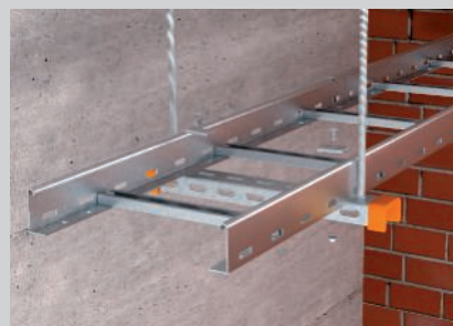
Mounting on transverse profile with clamping piece, truss-head bolts and large washers.
