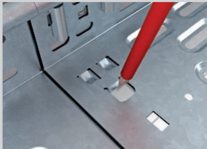
Bending the locking straps in the base.
